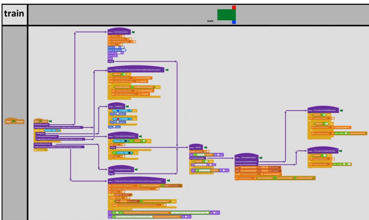
Figure 4. Modularization example inside the only scenario created with the use of procedure calls, across four hierarchy levels highlighting the tree structure
